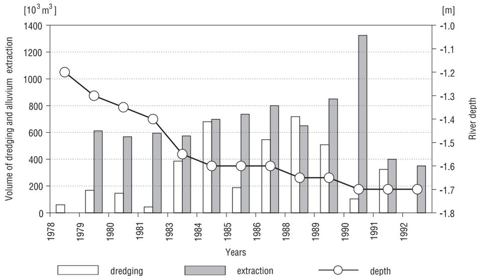
Figure 2. Correlation between the volumes of dredging and alluvium extraction and river depth
