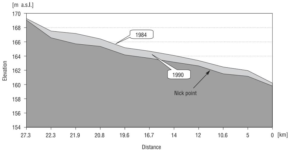
Figure 4. The Katun' River longitudinal profile in navigable reach by low water
