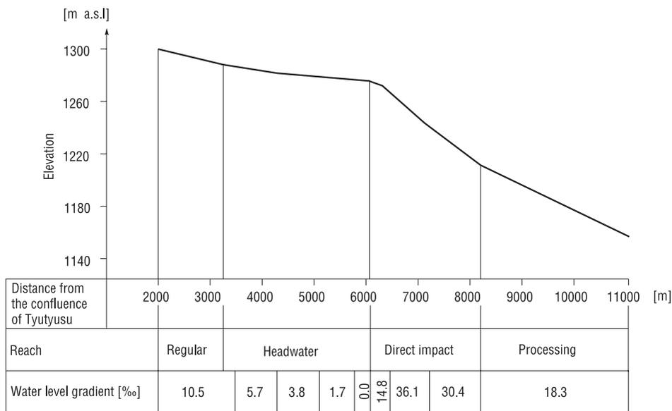
Figure 2. Baksan longitudinal profile near the town of Tyrnyauz after catastrophic valley debris-flows on the Gerkhozhansu, 18-25 July 2000
