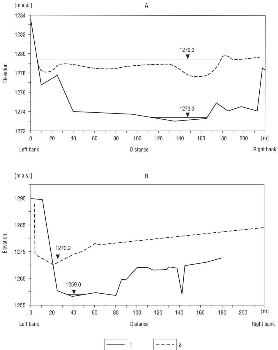
Figure 3. Near-channel cross-sections of the Baksan valley
